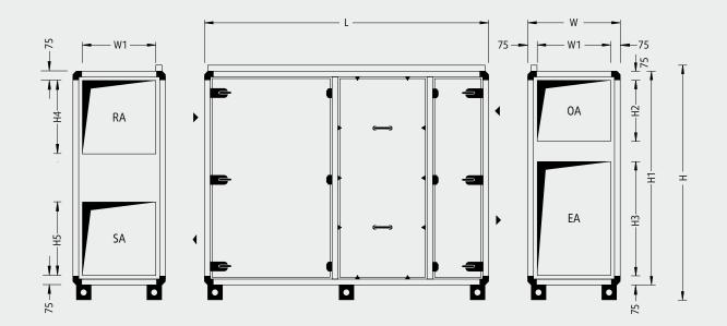
Important! Where a system is operated in parallel, the supply air and return air ducts of the two units have to be brought together.
